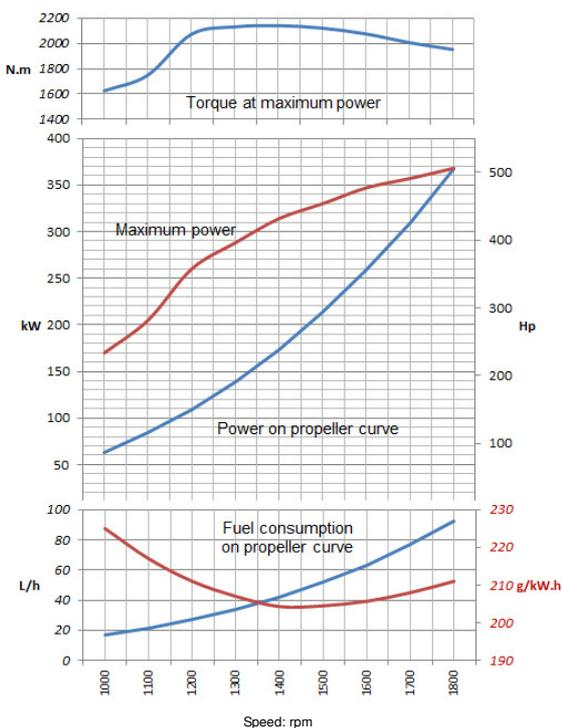
P2 rating - 404 kW / 550 hp @ 1900 rpm
